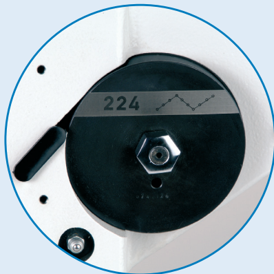
Easily inter-changeable cams
