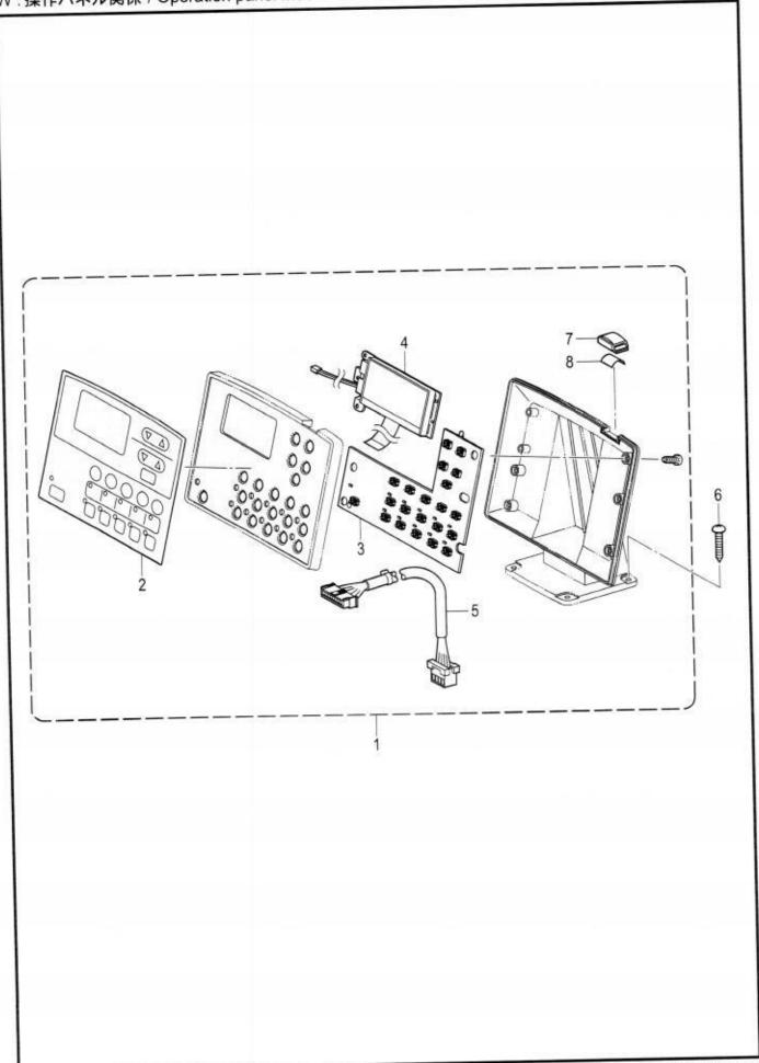
W. 操作パネル関係 / Operation panel mechanism
