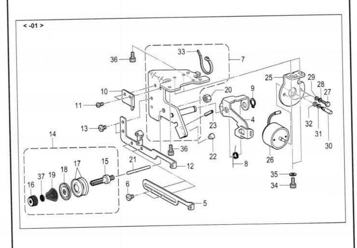
P2. 糸通し関係 / Threading mechanism
