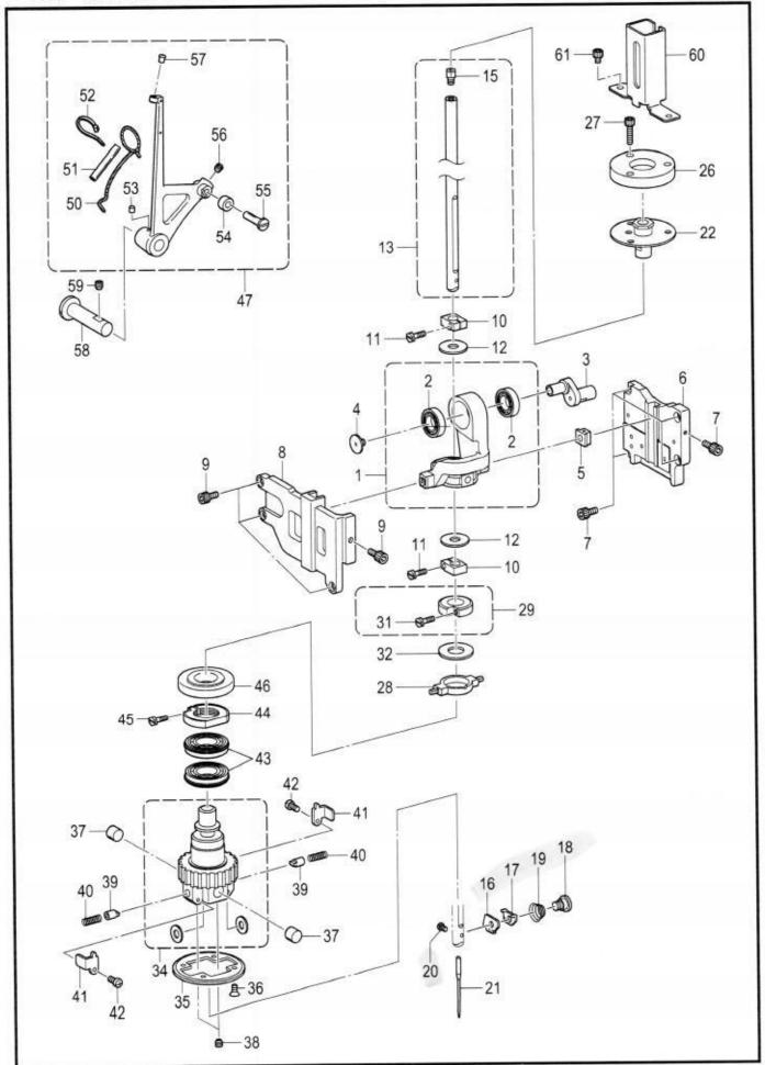
B. 針棒・天秤関係 / Needle bar and thread take-up mechanism
