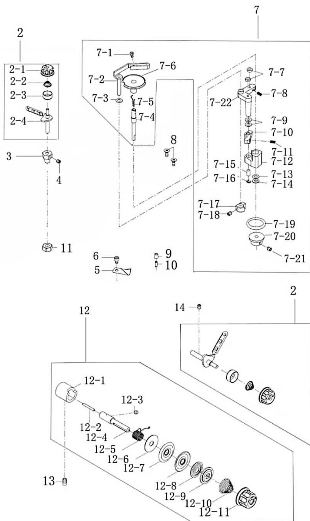
B. Bobbin winder and thread tension parts
