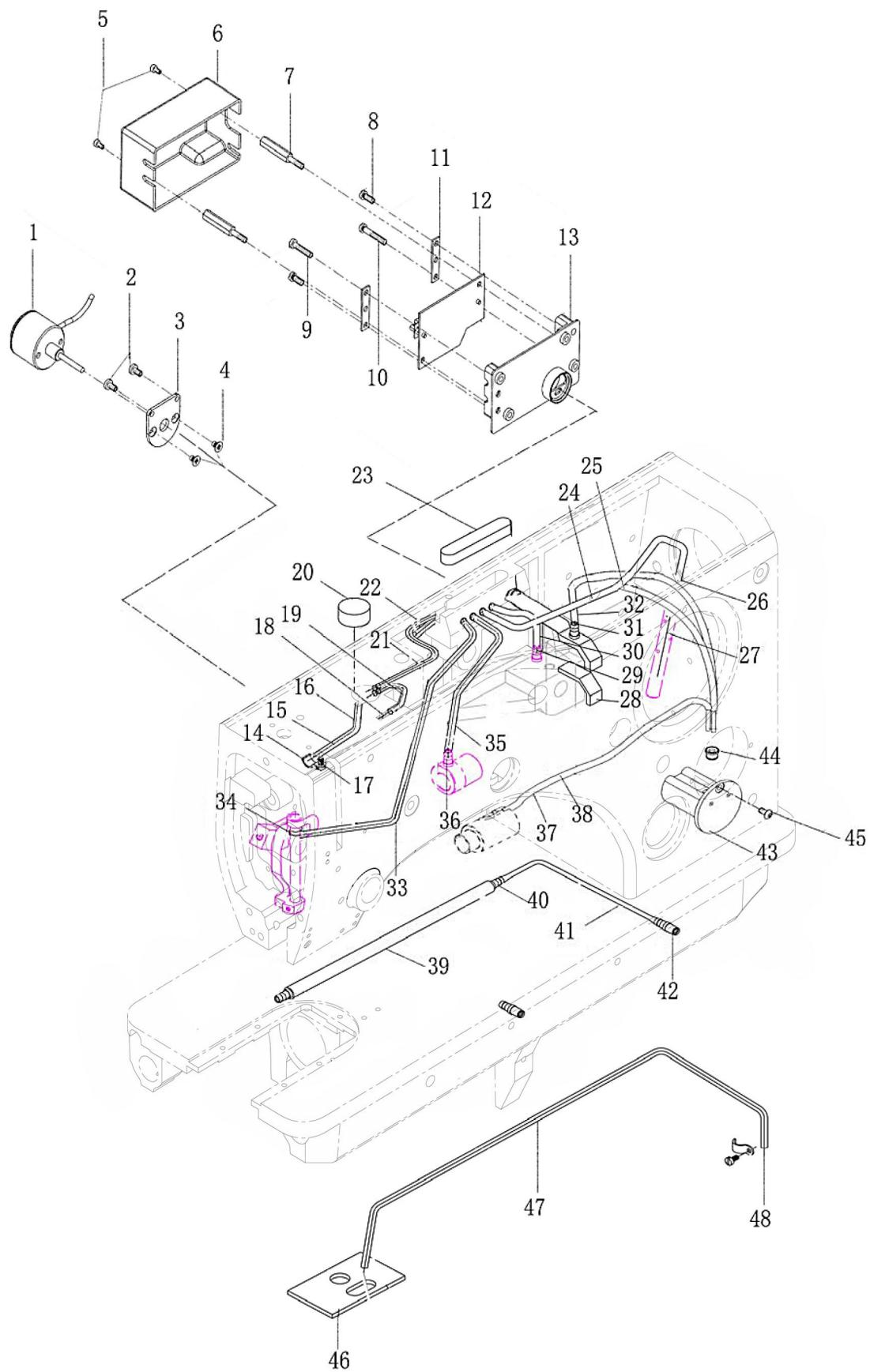
M. Tension release, electrocircuit board, oil circuit parts
