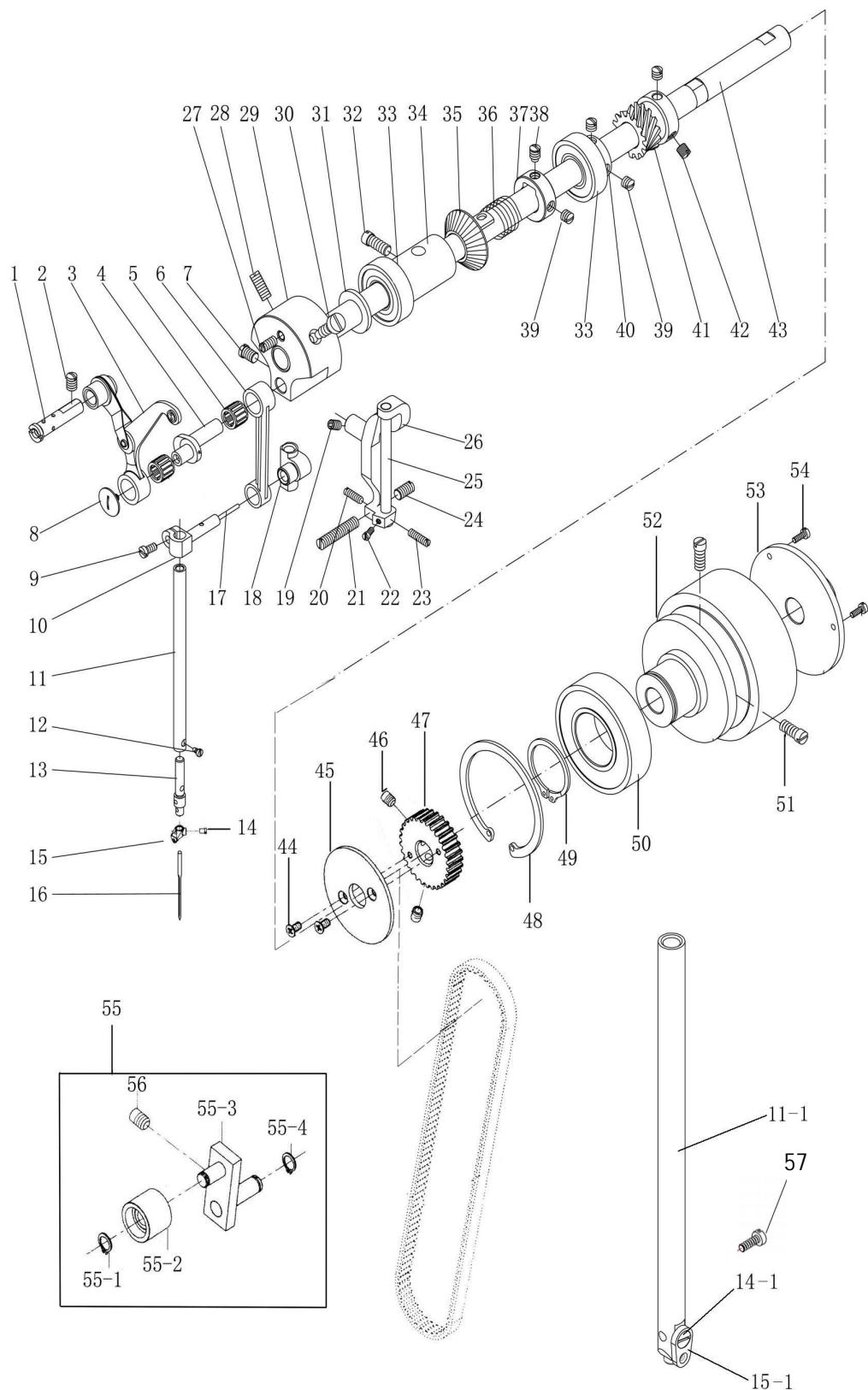
C. Arm shaft and needle bar thread take up parts
