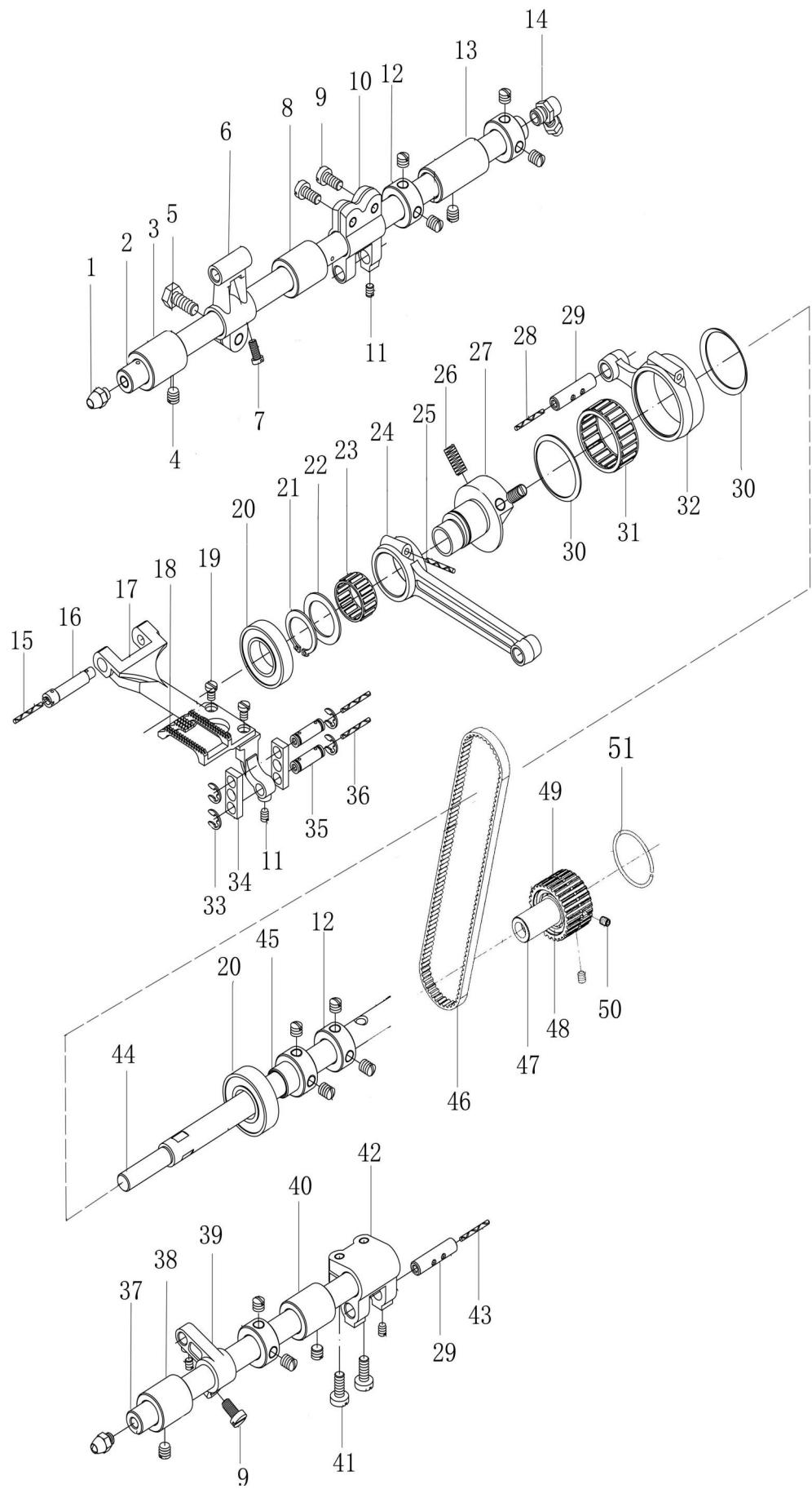
H. Lower shaft, feed dog and presser foot lifting parts
