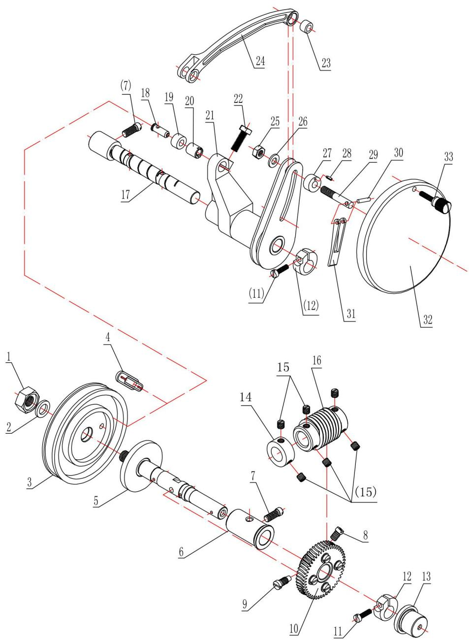
O. Special parts for cam patterns zigzag machine
