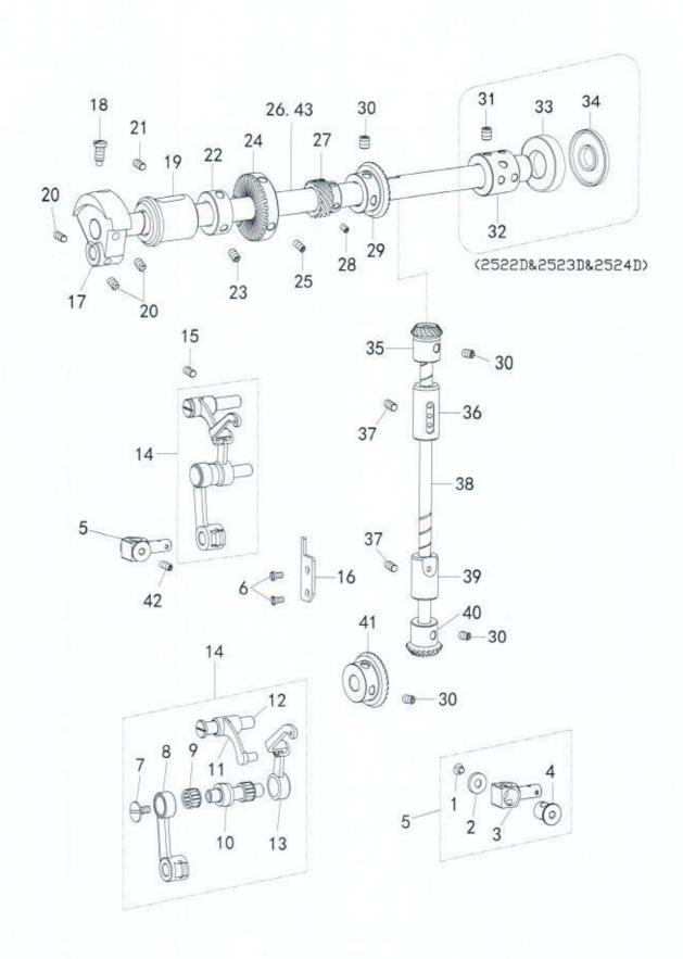
2. 上轴. 竖轴. 挑线机构/Upper shaft mechanism
