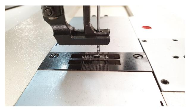
The feed dog is at its topmost point when the needle is at its lower dead point (see picture below).
