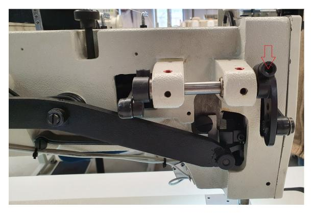
The lifted foot will be lowered by the presser foot spring down to the throat plate.
