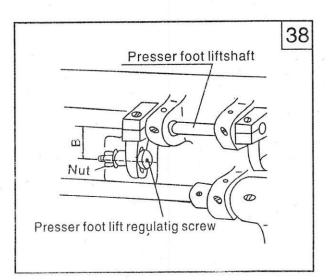
6.5 Adjusting the top feed mechanism 6.5.1 Gc2301
