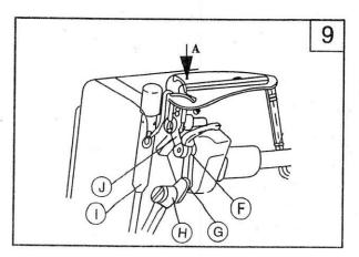
Oil applied to hole A is distributed to parts F, G, H, I and J through oil wick (fig.9)
