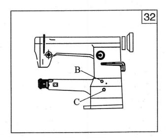
When adjusting the feed dog, first remove sliding ring. guard ring .needle, and make feed dog raised to highest position. Insert screwdriver into hole B to loose feed rockshaft crank clamping screw slightly and move the feed bar to adjust the height of the feed dog Tighten clamping screw after proper height of feed dog obtained. (Fig. 32)
