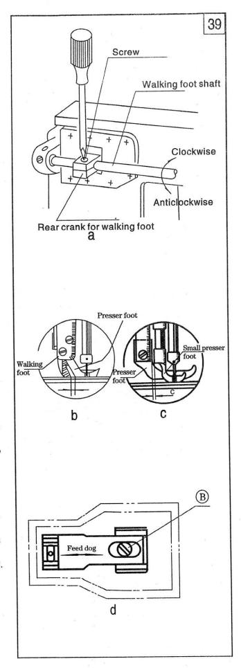
If the needle penetrates right or left into the center point of the hole, adjustment can be made as this:loose setscrew B (fig.39.b) and adjust position of feed dog. Tighten screw B after adjustment.
