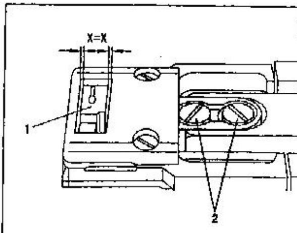
2. Positioning the feed dog in the direction of sewing(Fig.12)
