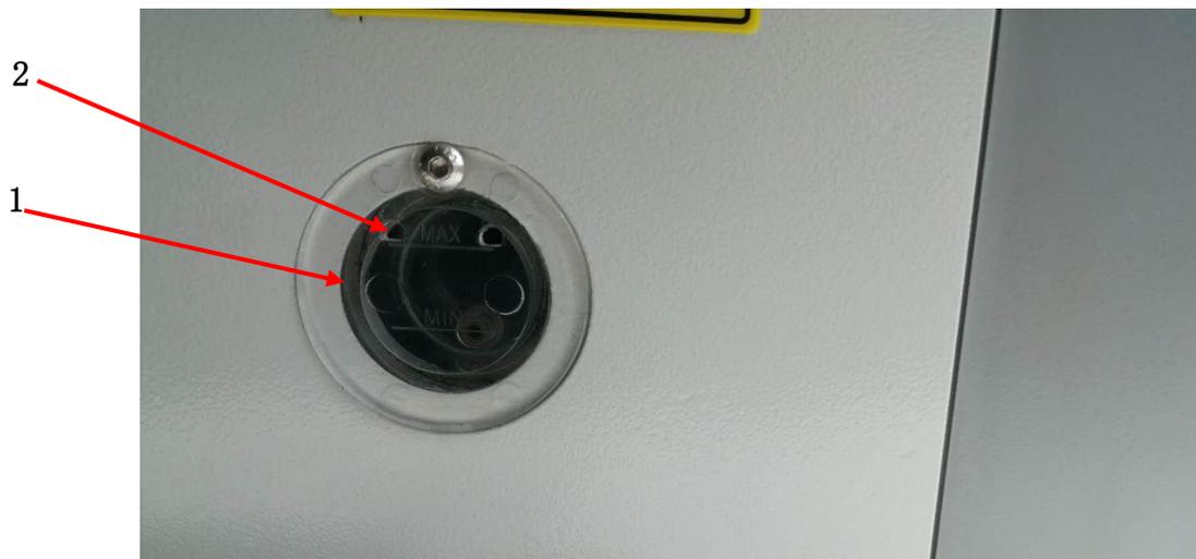
Check the oil level before each use. There must always be oil in reservoir **1**.
