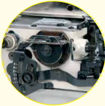
External adjustment differential feed mechanism
