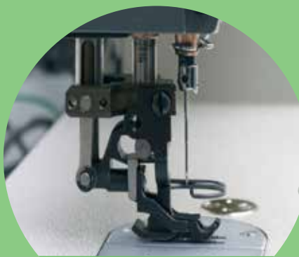
TOP FEED PRESSER FOOT MECHANISM
