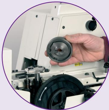
The cams of the BH 1000 are easily interchangeable; just remove and replace
