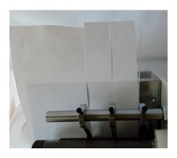
Now tightly screw the nut under the serrated nut with wrench 17, please pay attention that the screw cannot turn downward anymore, this will withheld the knife from cutting the paper/leather.
