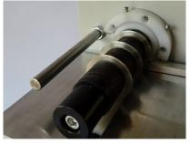
Now lower the nylon pressure roll by unscrewing the lower bolt with a wrench, after this keep turning the hand wheel until the nylon roll is detached from the blade.
