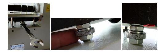
As soon as the blades are detached from the nylon roll you take the big allen-key and twist the closure cap (<u>clockwise</u>) from the knife spindle until it comes loose.
