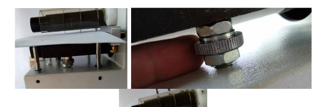
Now you need to test it, pay attention if the knives are cutting the paper properly. If this is not the case, gradually twist the serrated nut to the left while stopping now and then to see if the paper is being cut.
