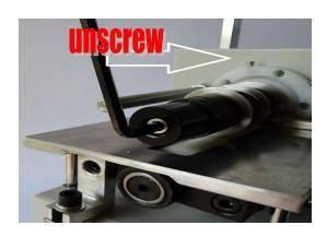
Before unscrewing the knife spindle cap, you can block the spindle with a screwdriver.
