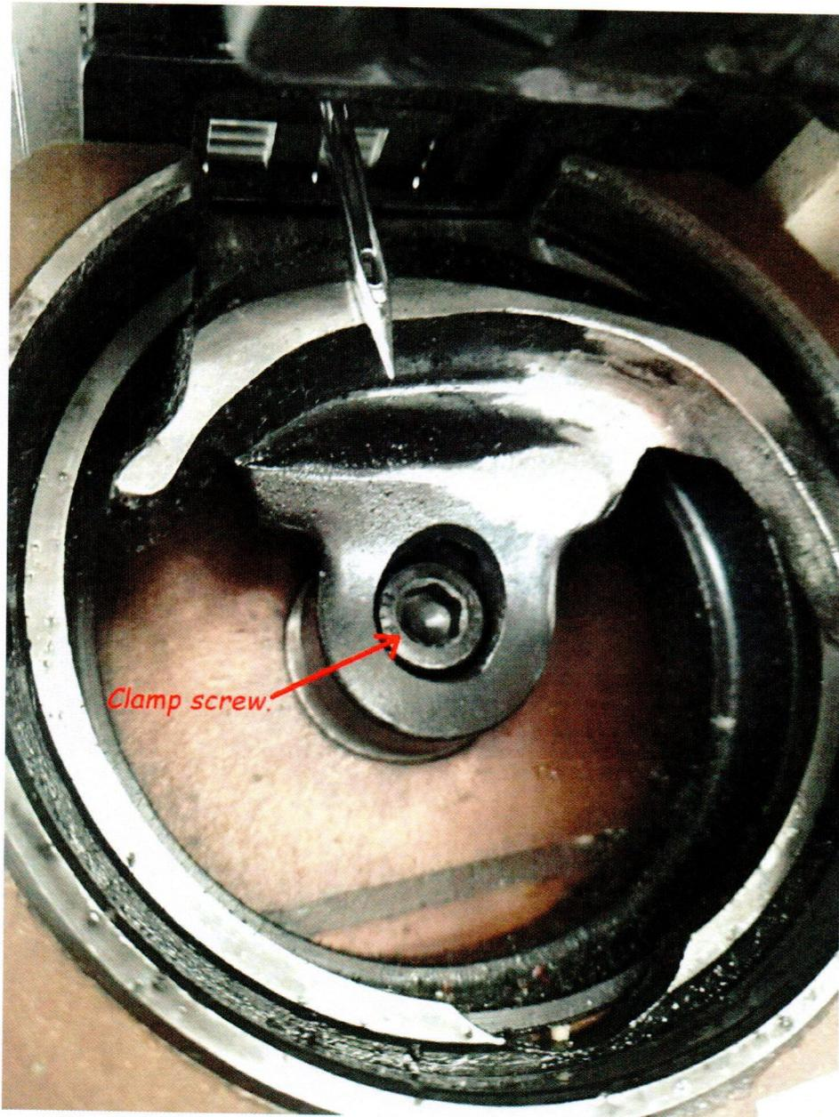
*Remove shuttle driver clamp screw & shuttle driver. Inside where shuttle driver fits are spacing washers. Either add or remove washers to set driver to guard needle as required.*
