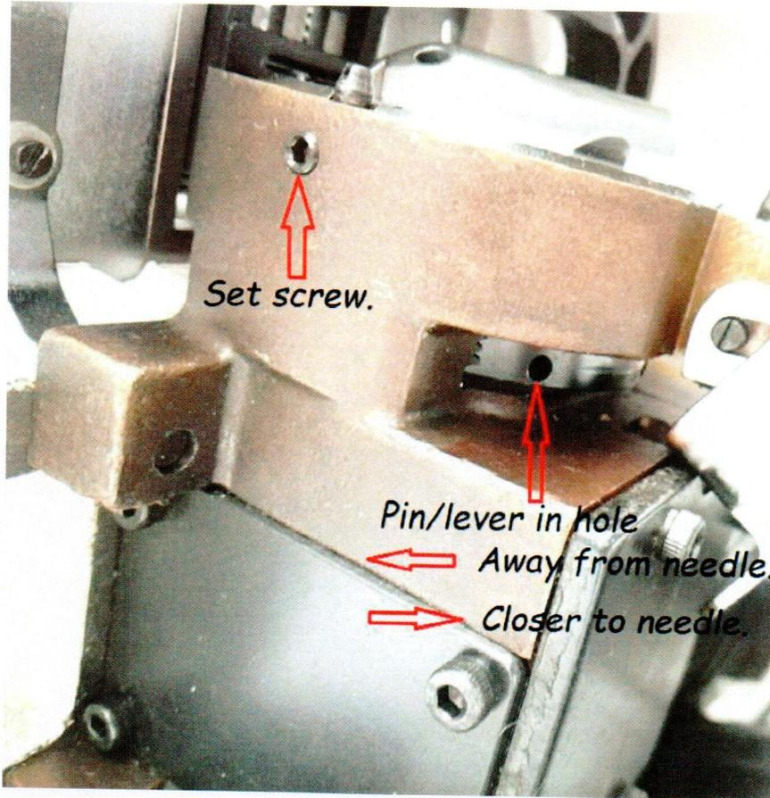
Loosen set screw. With a pin/lever adjust race to needle.
