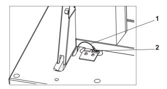
The earth (grounding) cable (1) is included in the machine's accessory pack.
