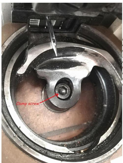
Remove shuttle driver clamp screw & shuttle driver.
