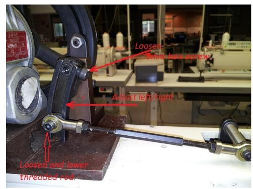
Lower threaded rod to make wide zig zag. Loosen 5mm hex screw and adjust lever left or right to centralise needle on wide zig zag.
