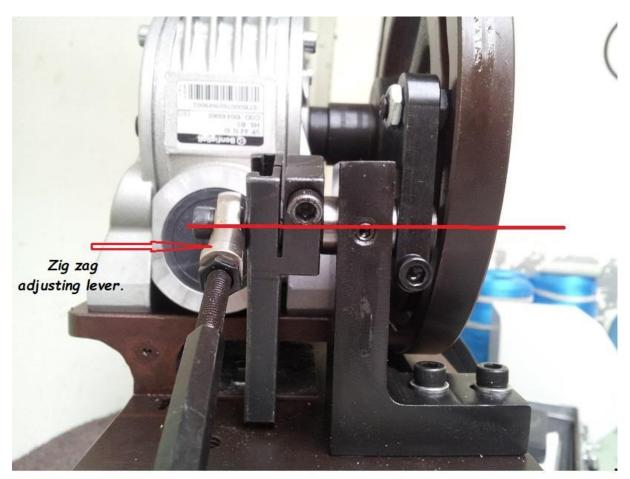
First, you must make the zig zag adjusting lever to zero (straight stitch).
