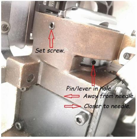
Loosen set screw. With a pin/lever adjust race to needle.
