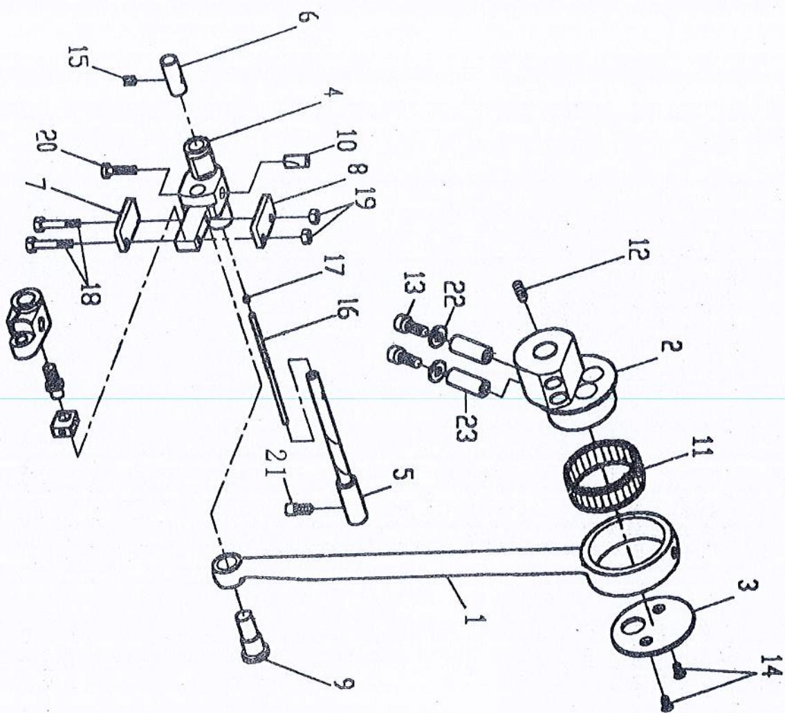
F、下轴机构 HOOK DRIVING SHAFT COMPONENTS (2/2)
