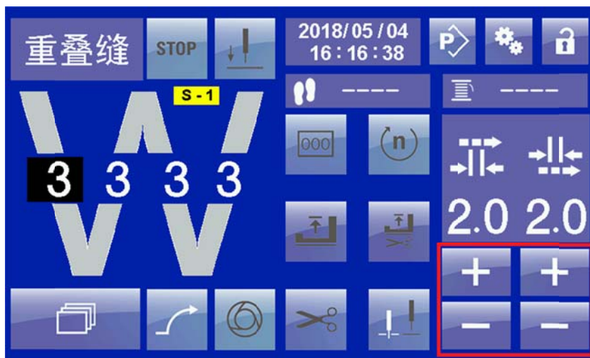
9 Overlapping sewing interface - scroll value setting
