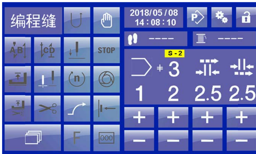
11 Programmed sewing interface- multi-segment shift
