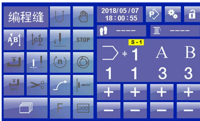
12 Programmed sewing interface- setting start back-tacking
