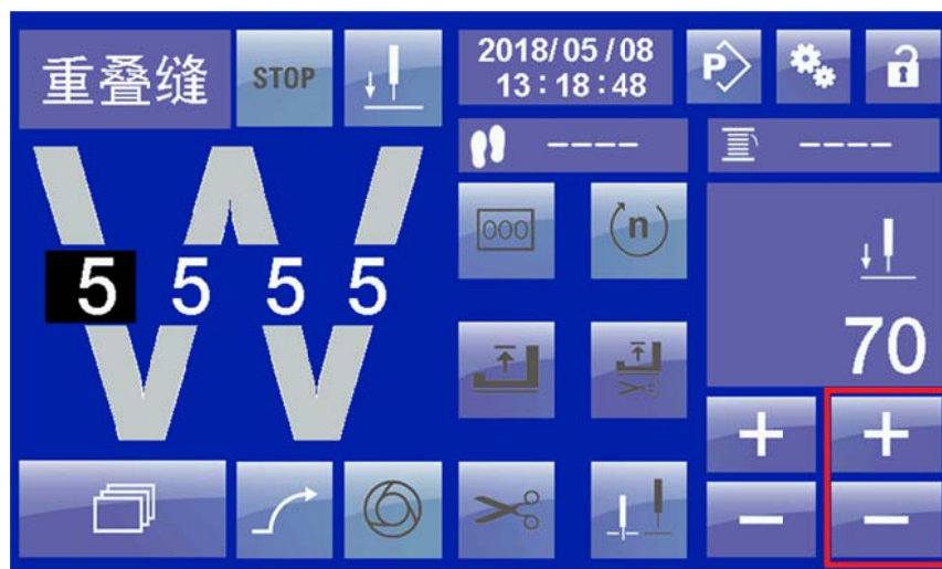
10 Overlapping sewing interface- needle position setting
