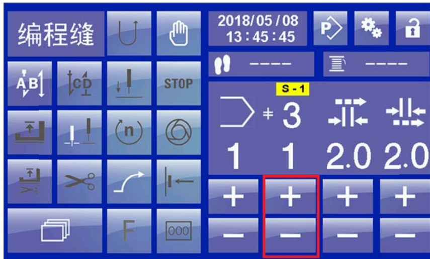
10 Programmed sewing interface - multi-segment shift
