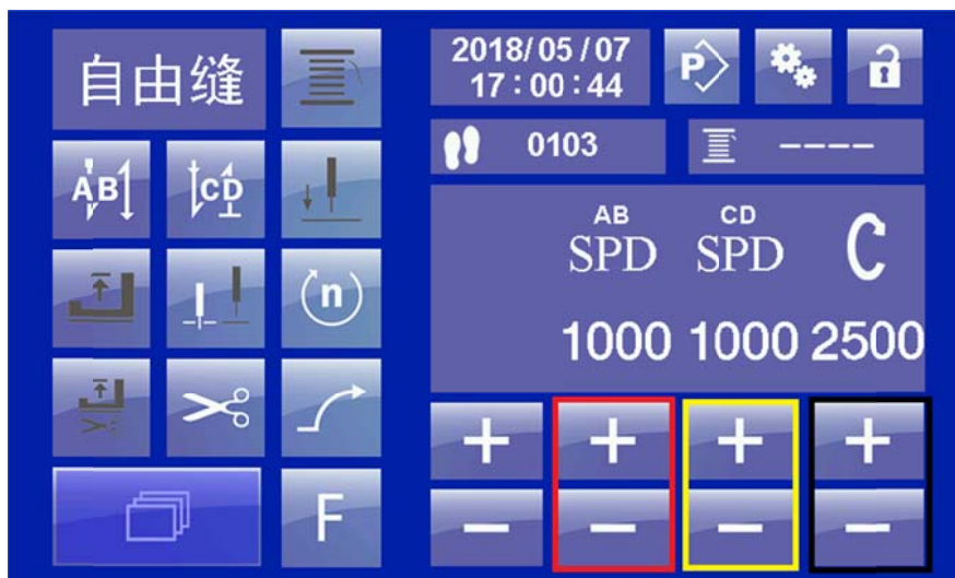
7 Free sewing interface - speed setting
