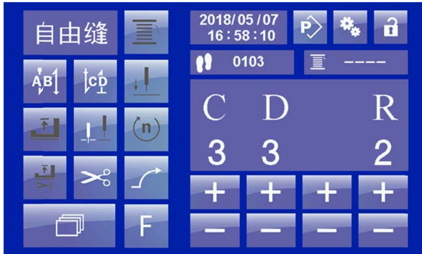
6 Free sewing interface- End back-tacking setting
