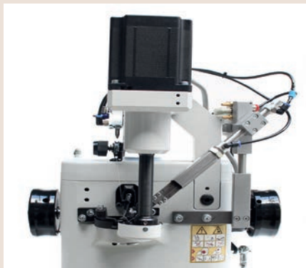
Pneumatic thread trimmer (option).
