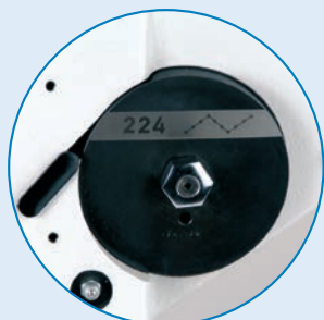
Easily inter-changeable cams
