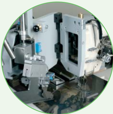
Head tilted back for quick and simple servicing and maintenance.
