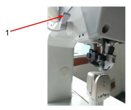
• The roller presser can be raised by turning lever **1**.
