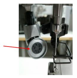
When the roller presser is raised, it can be swung out by pulling it lightly downwards (see arrow).
