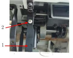
Fix the tilt lock **1** by screw **2**. (Supplied with accessories)
